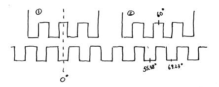
From the figure, we see that if phase 1 is turned off and phase 2 is energized, the rotor will rotate  $4.61^{\circ}$  degrees to the right (clockwise) to align with the phase-2 pole. Similarly, if phase 3 is excited after phase 1 is turned off, the rotor will rotate  $4.61^{\circ}$  degrees to the left (counterclockwise).
