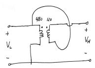
part (b): The rated current of the high voltage terminal is equal to that of the 120-V winding,  $I_{\text{rated}} = 10^4/120 = 83.3$  A. Hence the kVA rating of the transformer is  $600 \times 83.3 = 50$  kVA.
