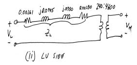
part (b): Following methodology of Problem 2.11, (i) for a power factor of 0.85 lagging,  $V_{\rm H}=4956$  V and (ii) for a power factor of 0.85 leading,  $V_{\rm H}=4000$  V.
