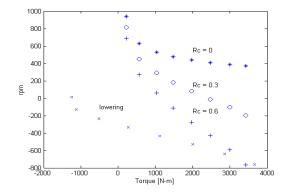
Operation in the fourth quadrant means that the motor torque is positive while the speed is negative. In this case the motor is acting as a generator and absorbing energy from the lowering load, which would otherwise accelerate due to the effects of gravity.
