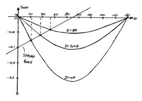
part (e): The curve of spring force versus angle is plotted as a straight line on the plot of part (d). The intersection with each curve of magnetic force versus angle gives the equilibrium angle for that value of current. For greater accuracy, MATLAB can be used to search for the equilibrium points. The results of a MATLAB analysis give:
