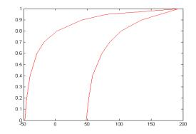
part (b): Area = 191 Joules part (c): Core loss = 1.50 W/kg.
