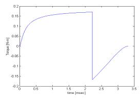
The integral under the torque curve is  $2.38 \times 10^{-4}$  N·m·sec while the positive torque integral is 3.29 N·m·sec. Thus there is a 25.7% reduction in torque due to negative torque production during the current-decay period.
