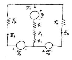
$$\mathcal{R}_{A} = \frac{l_{A}}{\mu A_{c}}; \quad \mathcal{R}_{1} = \frac{l_{1}}{\mu A_{c}}; \quad \mathcal{R}_{2} = \frac{l_{2}}{\mu A_{c}}; \quad \mathcal{R}_{g} = \frac{g}{\mu_{0} A_{c}}$$
