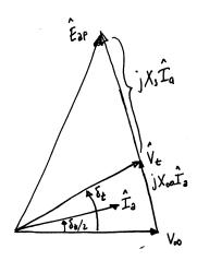
(ii)  $V_{\rm t}=V_{\infty}=1.0$  per unit. P=375/650=0.577 per unit. Thus
